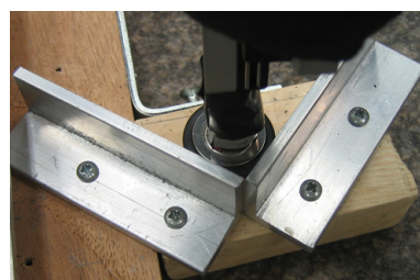
Fig. 9. Photograph of robot endpoint in contact with hold designed to simulate friction.
